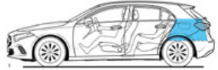
Open luggage compartment behind rear seat, loaded to upper edge of rear seat backrest, volume 310 litres (V 211-2)
